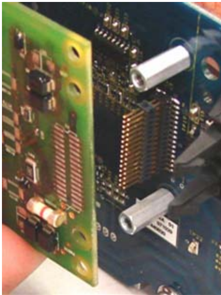
Figure 7 Installing new Fieldbus board
